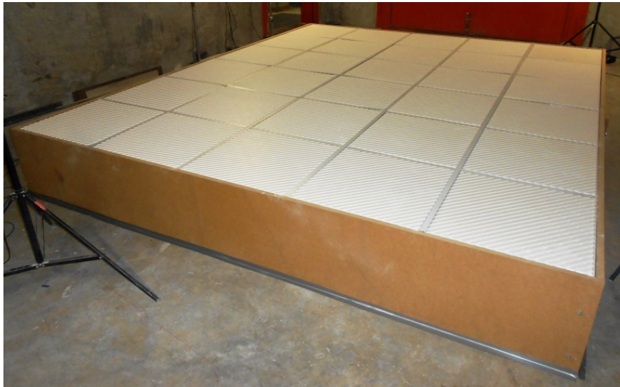
Figure 3: Bailey Interiors Nu TR2000 600mm x 600mm Perforated Plaster Ceiling Tiles with Sorbertextile P44FR acoustic fabric adhered to the underside of the tile tested with a 400mm air gap installed in Reverberation Room for testing.
