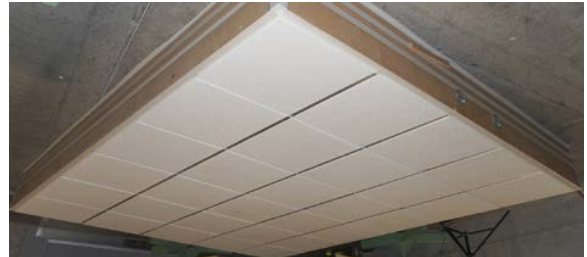
Test specimen installed for testing (image inverted to depict ceiling installation)
