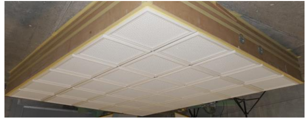
Test specimen installed for testing (image inverted to depict ceiling installation)
