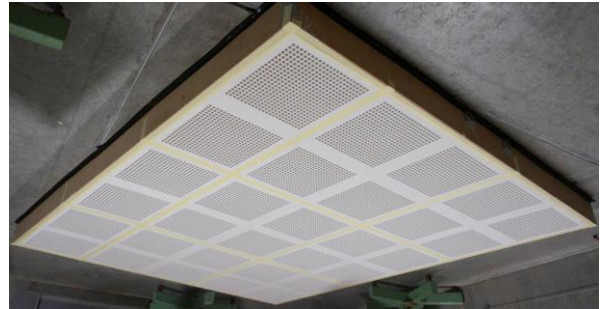
Test specimen installed for testing (image inverted to depict ceiling installation)
