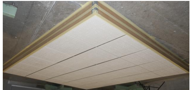
Test specimen installed for testing (image inverted to depict ceiling installation)
