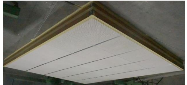
Test specimen installed for testing (image inverted to depict ceiling installation)
